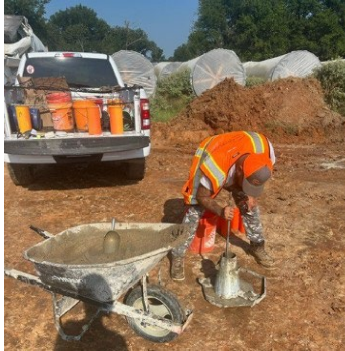
Concrete Slump Testing
