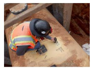
Coating adhesion testing
