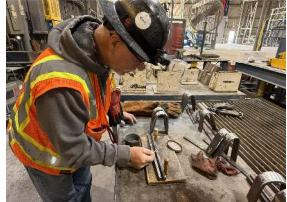
Pipe spiral weld testing
