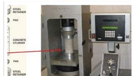
Concrete cylinders and compression strength testing
