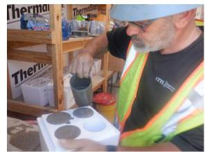
Concrete and grout compressive strength testing
