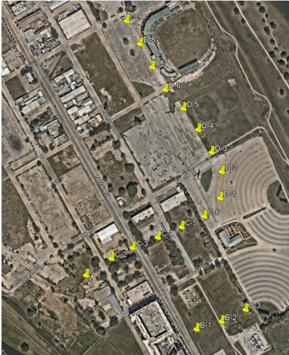
Figure 3: Geotechnical boring locations
