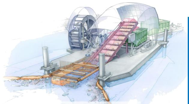
The waterwheel measures 52' long, 24' wide with a wheel that is 14' in diameter and 3' wide.
