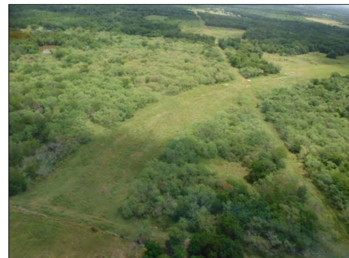
PL1718 Aerial photos of pipeline ROW restoration
