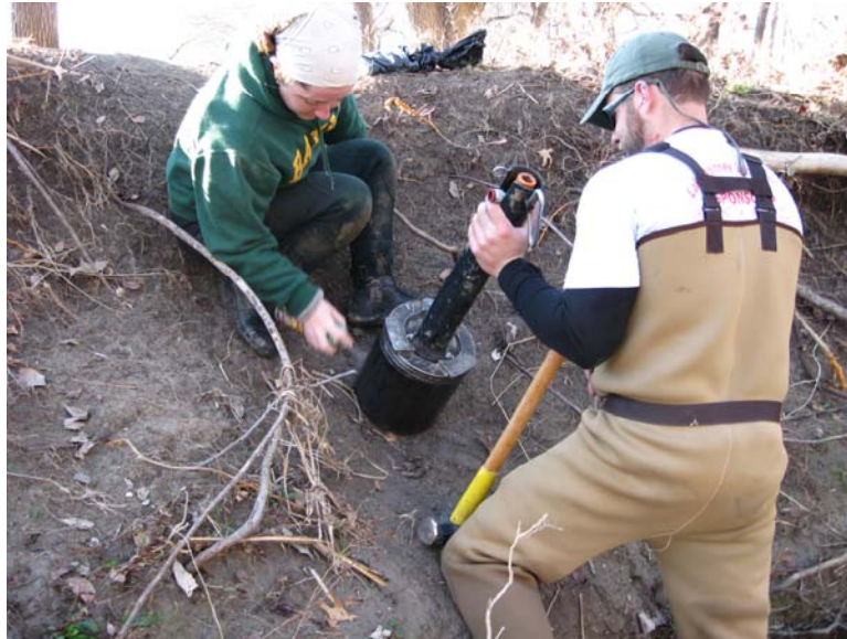
Figure 10. Photograph of the 20.3 x 20.3 cm, 6.35 mm steel tube with pneumatic extraction being placed on the upper bank to collect a soil sample for laboratory for submerged jet testing.
