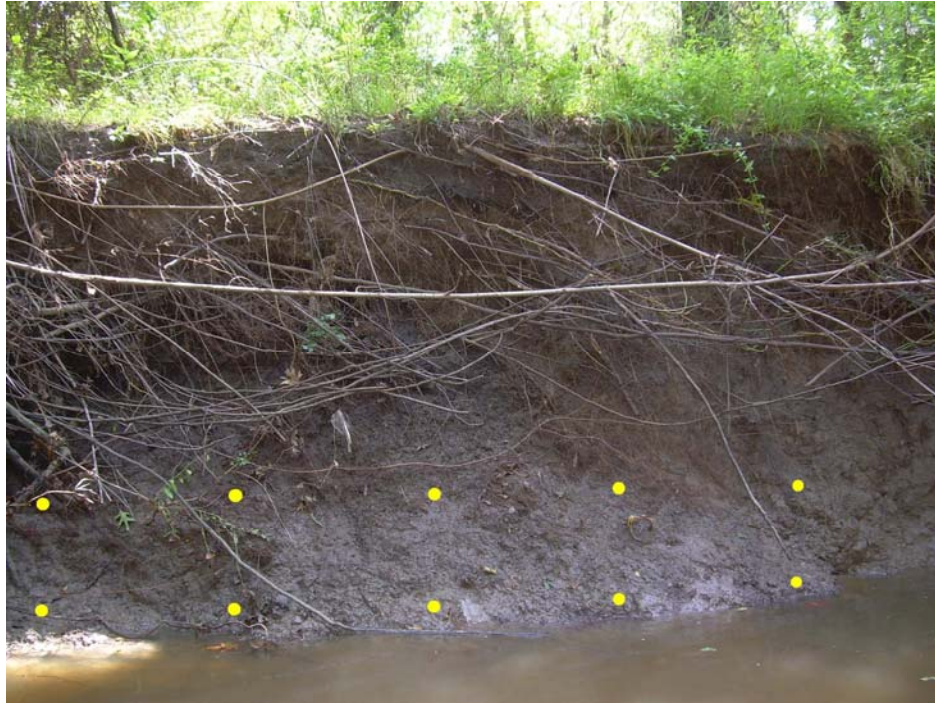
Figure 8. Photograph of the upper and lower bank erosion pin locations shown in yellow, spaced 1 m apart after Zaines et al. 2005.
