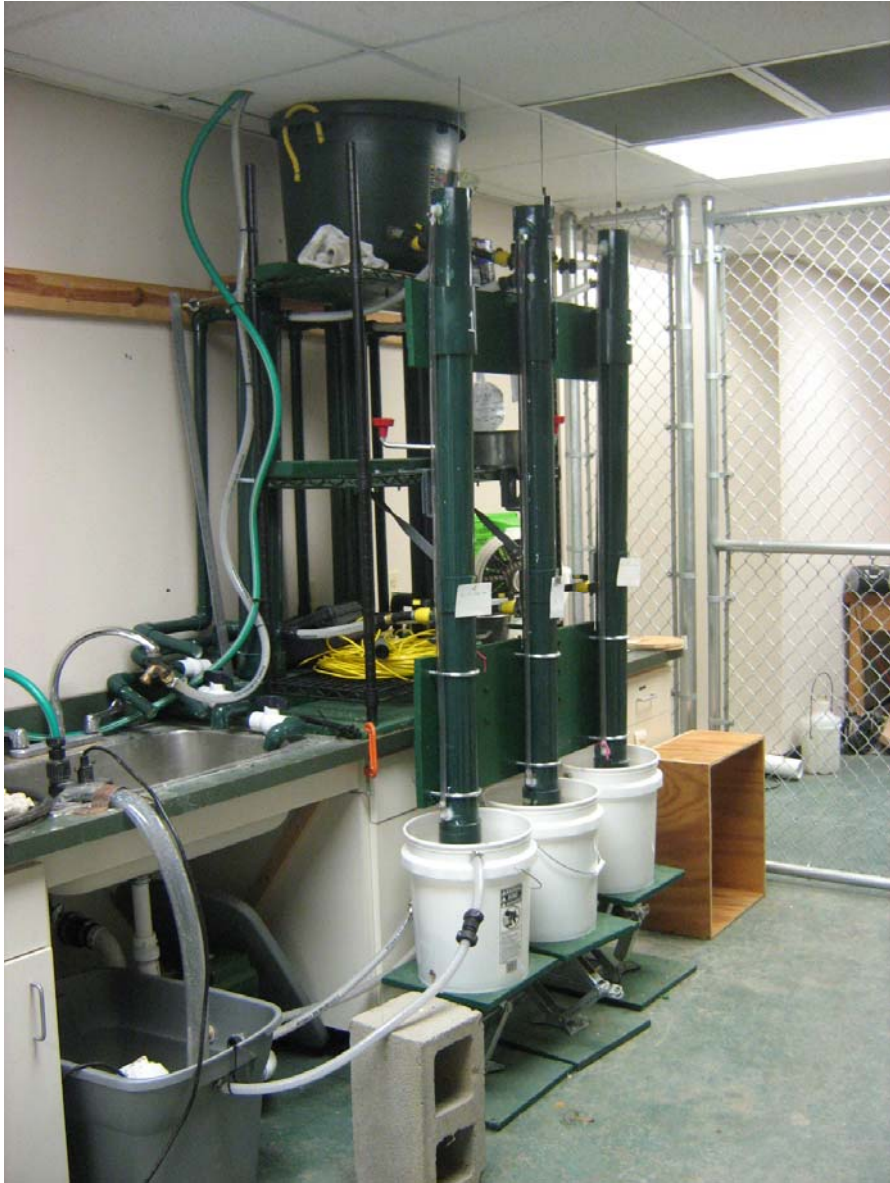
Figure 12. Photograph of the in-lab submerged jet test device (modified by Allen, Capello, and Coffman) during testing of three soil cores from the study area.
