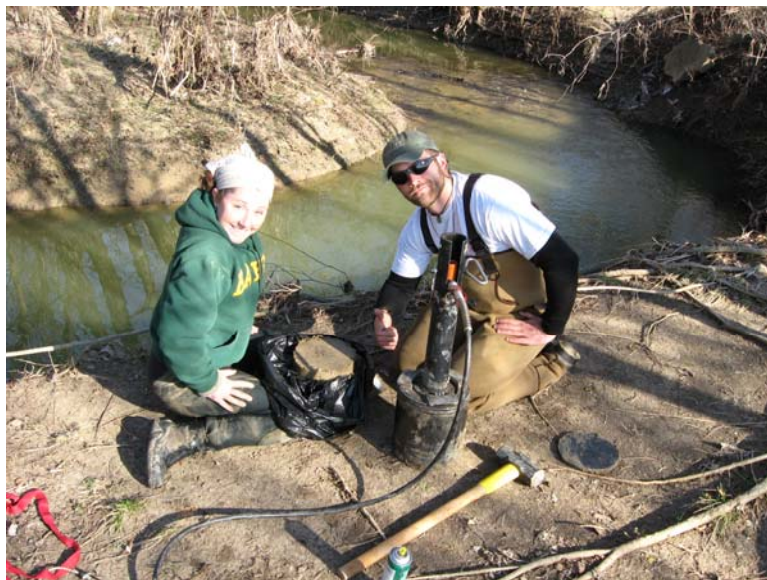
Figure 11. Photograph of the 20.3 x 20.3 cm, 6.35 mm steel tube with pneumatic extraction next to an extracted soil sample, being carefully prepared for transport back to the laboratory for submerged jet testing
