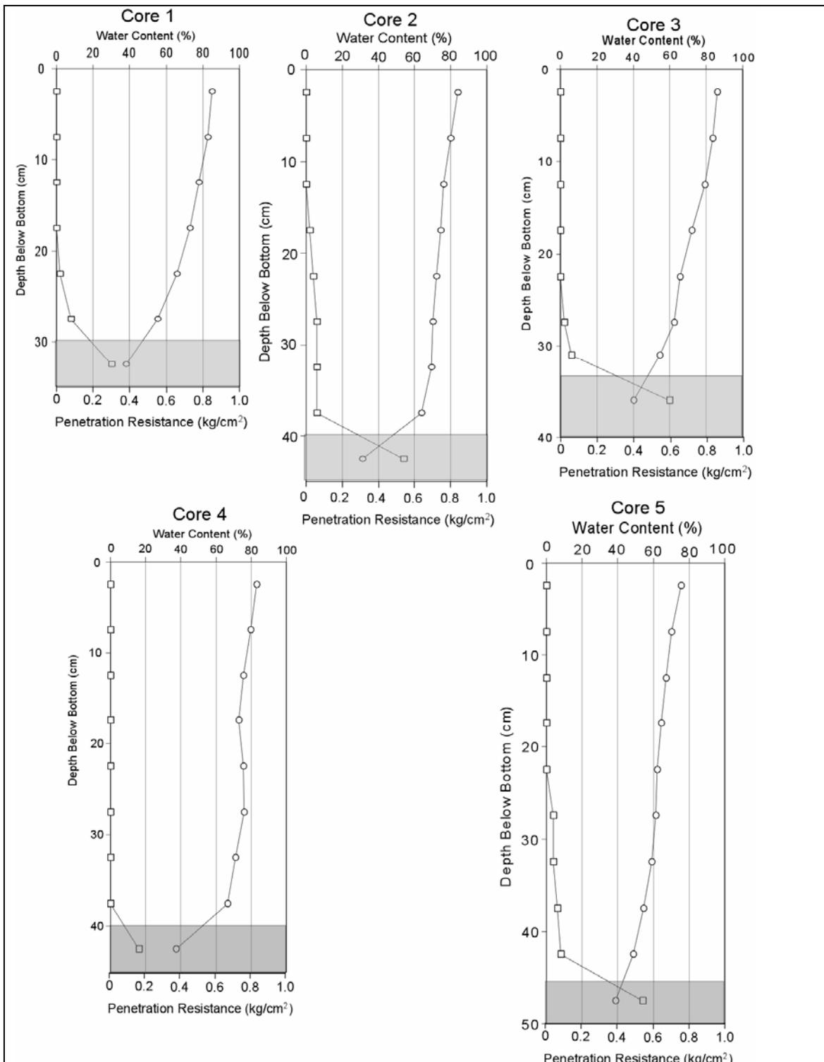
Figure 3. Water content and penetration resistance in cores collected in Cedar Creek Reservoir. Circles mark the variation in water content by weight. Squares mark the variation in penetration resistance. The regions of the graphs with white background correspond to the post-impoundment sediment. The regions with gray background correspond to the underlying pre-impoundment soil.
