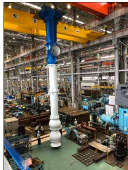
OFE09 Pump assembly for JCC1 vertical pump in Japan
