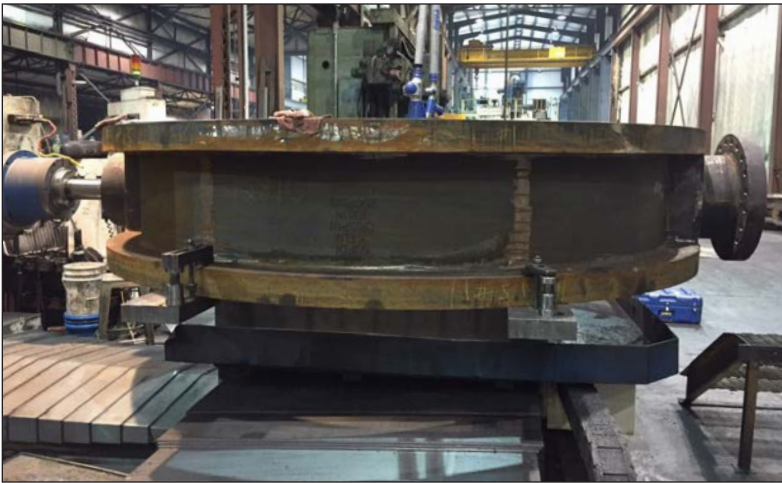
Machining of 108-inch Butterfly Valve Body at Davis Machine and Fabricating, Calera, AL
