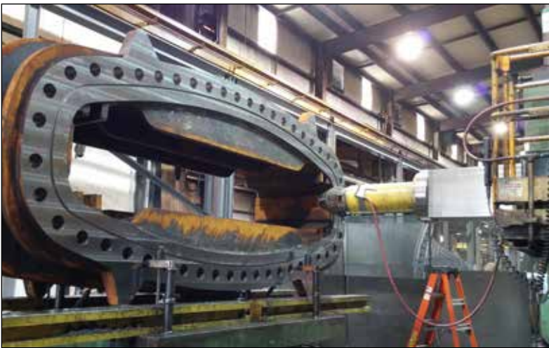
Machining 108-inch-diameter gate valve intermediate body section at JTL Integrated Machine, Port Colburne, Ontario
