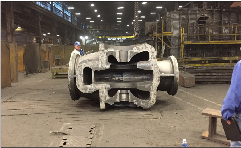
JB3 Factory inspection of pump bottom casting in Cincinnati, Ohio
