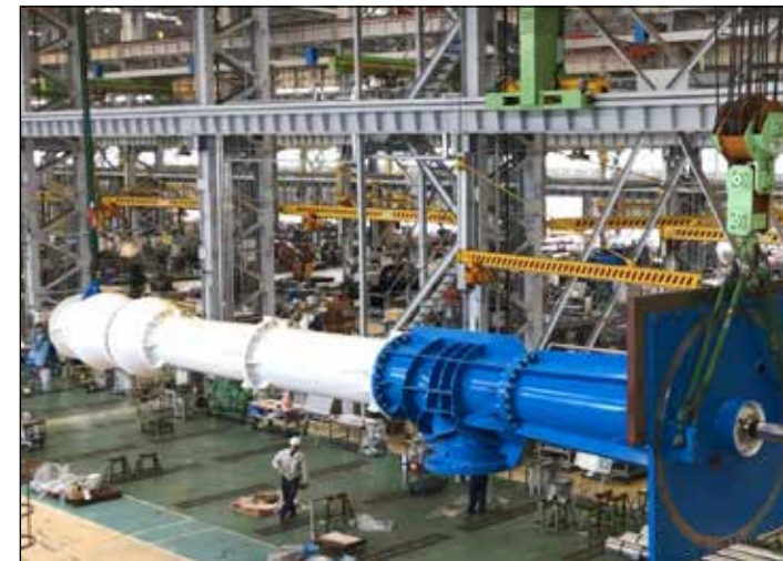
OFE09 Preparing for performance testing of JCC1 Pump 2 in Japan
