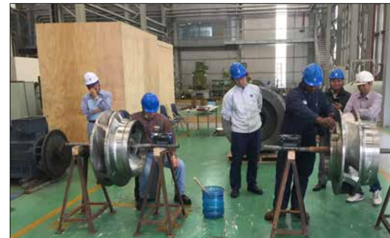
OFE09 Performing ultrasonic testing of pump impellers in Vietnam
