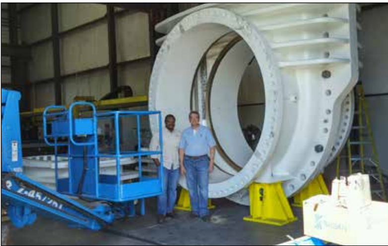
OFE03 Partially assembled 108-inch gate valve
