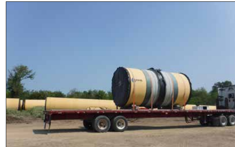
PL1718 Receiving monolithic isolation joint
